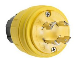
Locking Watertight Plug, 30amp 125/250volt, NEMA Configuration L14-30, multipoint sealing system provides environmental protection of: NEMA 4, 4X, 6, 6P and IP67 rated.
