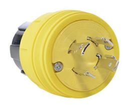
Locking Watertight Plug, 30amp 3 480 volt, NEMA Configuration L16-30, multipoint sealing system provides environmental protection of: NEMA 4, 4X, 6, 6P and IP67 rated.
