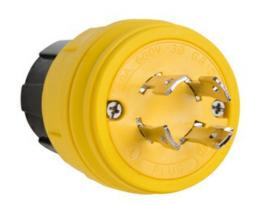
Locking Watertight Plug, 30amp 3Y 600volt, L17-30 configuration, multipoint sealing system provides environmental protection of: NEMA 4, 4X, 6, 6P and IP67 rated.
