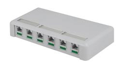
Ortronics 6 port high density jack (HDJ) Surface Mount Outlet Box accept 6 jack modules and provides snap-on covers and snap-in label fields. 6.98" x 4.33" x 1.16". Box is supplied with screws and double-sided adhesive tape for mounting onto almost any surface.
