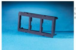
This plate accepts three TracJack modules or blanks. Use with 40700071, 40700072, or 40700073 bezels, to snap mount into 2.70'' x 1.375" TIA referenced furniture openings for Steelcase, Haworth, Knoll and others. 5 pack.
