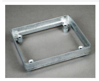
1"" (25mm) high extension. Used to increase height of preset or afterset. Die cast construction. Attach to preset or afterset with push on metal sleeves (included). Can be stacked.
