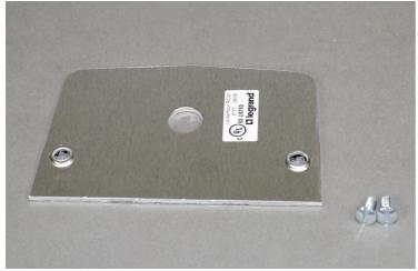
Single receptacle faceplate. Hole diameter: 1.0625" (27mm). NOTE: Four-piece service fittings include: housing and base plate. Receptacles included when indicated in part number description. 525 Series Service Fittings have 27 cubic inches (442ml) of capacity.
