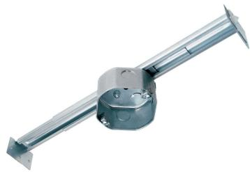
Slide fan support - same heavy-duty slide as 55501, but with 2.0-inch deep box, to accommodate up to 1-inch firewall or soundproofived ceilings, with rotating dual support for 16-24-inch spans, bulk packed. 25-Pack.
