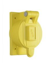
All Pass and Seymour weatherproof covers are built tough to endure the harshest weather conditions. This model includes a vertical self-closing flip lid that prevents contaminants from entering the device. Complete with stainless steel screws, it is completely corrosion resistant. Multiple gaskets are provided to ensure a tight seal and easy installation. The molded label area allows you to appropriately label the outlet for quick identification.
