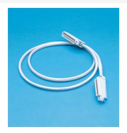
Legrand® voice 25-pair cable assemblies are constructed from 24 AWG solid conductor UTP cables terminated with industry standard 50-pin telco connectors.
