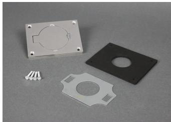
Brushed aluminum single locking receptacle cover plate. Single flip lid cover for 20A or 30A single locking receptacles. Device opening is 2 5/8" (67mm). For use with maximum female locking device of 1.58" diameter, and maximum male plug face of 2.25" diameter. NOTE: Brass covers and flanges are not interchangeable with aluminum or nonmetallic covers and flanges. Nonmetallic covers are interchangeable with aluminum flanges.
