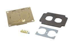
Brass duplex cover plate, for OmniBox® and Modulink™ Series floor boxes. Cover plate is 3.156 inch x 4.182 inch [80.2mm x 106.2mm]. Flip lids can also be used with 106 type frames for communications. NOTE: Brass covers and flanges are not interchangeable with aluminum or nonmetallic covers and flanges. Nonmetallic covers are interchangeable with aluminum flanges.
