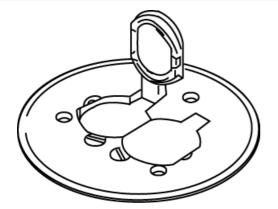
The Wiremold Ratchet-Pro<sup>™</sup> brass duplex cover plate with flip lids, 5 1/2 inch (140mm) for carpet or tile installations. NOTE: All cover plates are furnished with gasket and three screws.
