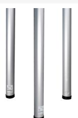
Satin anodized finish. Nominal wall thickness .060" (1.5mm). Length: 10' 3" (3.1m). Provided with one 1/2" (12.7mm) trade size KO at base. T-bar mounting hardware, ceiling trim kit, foot assembly, and grommet included. Feed box not furnished.
