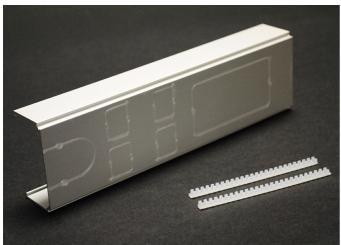
For AMDTP-4 and AMTC-4 Series. 8" (203mm) long. Communication covers for additional voice/data connectors. Each cover includes KOs for four RJ11/RJ45 connectors (.760" x .576" (19.3mm x 14.6mm)), mouse hole for exiting communication cables (grommet furnished).
