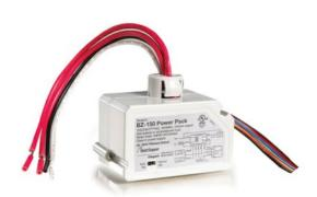
The BZ-150 Universal Voltage Power Pack is full featured and can provide 24 VDC operating voltage to Wattstopper's lowvoltage occupancy sensors. In addition, the BZ-150 enables manual-on, hold-on, hold-off and load shed applications when used with lighting control panels or building management systems. This device is constructed with environmentally friendly materials and is RoHS-compliant.
