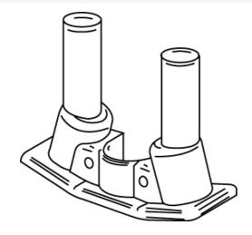
For two 3/4" trade size conduit connectors (no additional capacity).
