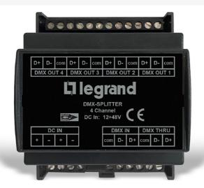
The Wattstopper DMX-SPLITTER is a repeater that divides and regenerates the DMX/RDM input signal into four output channels. It is used with DMX controlled lighting systems when the maximum of 32 devices per bus run is exceeded. In this way, more devices can be added to a DMX network without adding a new DMX-DALI controller. In addition to DMX, the DMX-SPLITTER also distributes RDM messages for devices that use RDM
