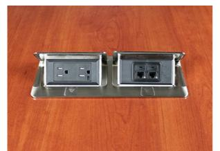
Unit includes one (1) 15A black tamper-resistant duplex receptacle. Second opening will accept adapter for one (1) Wiremold CM Series Open System 2A module, one (1) Ortronics Series II or one (1) TracJack adapter to accommodate a wide range of communication outlets. Adapters are included in hardware bag. Unit comes with a 6' (1.83m) cord. Comes with a brushed stainless steel finish.
