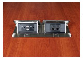
Unit includes one (1) 15A black tamper-resistant duplex receptacle with two (2) USB ports that provide 3.1A. Second opening will accept adapter for one (1) Wiremold CM Series Open System 2A module, one (1) Ortronics Series II or one (1) TracJack adapter to accommodate a wide range of communication outlets. Adapters are included in hardware bag. Unit comes with a 6' (1.83m) cord. Comes with a brushed stainless steel finish.
