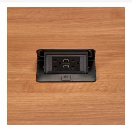
Unit includes one (1) 20A black tamper-resistant duplex receptacle with two (2) USB ports that provide 3.1A. Unit comes with a 6' (1.83m) cord. Comes with a black powder coat finish.
