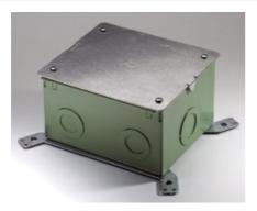
Evolution™ Series Furniture Feed On-Grade Floor Box is for use in on-grade and above grade concrete floor applications. Box is provided with a protective, disposable cover that allows the box to be installed at any point in the construction process. Box is available with an epoxy coating for on-grade applications. Custom options are available upon request. For use with carpet, tile and wood covered floors. NOTE: Not designed for use with bare concrete or terrazzo floors.
