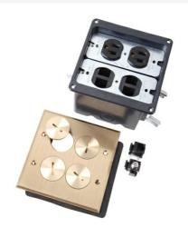
Tamper-Resistant Floor Box Assembly, Dual-voltage. Two #8 duplex openings, Four threaded screw plugs. Includes 3232 15A, 125A tamper-resistant duplex receptacle, Cat5E Jack, F-connector, Ten Blanks and a low-voltage dider. Brass. For detailed Tamper-Resistant receptacle information, visit our Tamper-Resistant Receptacles page.
