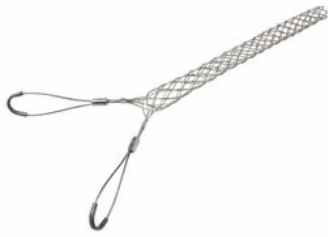
FC100UU: Standard Duty, Closed Mesh, Double -Eye Grip, Cable Diameter 1.00 - 1.24 inches, Bale Length 5-in, Mesh Length 15-in, Break Strength 1920 lbs.
