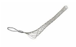
FC2000F: Standard Duty, Closed Mesh, Offset Eye Grips, Cable Diameter 2.00 - 2.49 inches, Bale Length 6-in, Mesh Length 22-in, Break Strength 3760 lbs.
