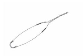
FC52: Bus Drop, Closed Mesh, Single Eye, Cable Diameter 0.53 - 0.73 inches, Bale Length 9-in, Mesh Length 6.5-in, Break Strength 1100 lbs.
