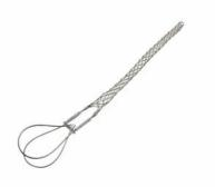
FCSD94LB: Service Drop, Closed Mesh, Locking Bale, Cable Diameter 0.94 - 1.25 inches, Bale Length 16-in, Mesh Length 11-in, Break Strength 1020 lbs.
