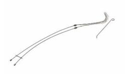
FR075LB: Standard Duty, Split Rod, Locking Bale (Universal Eye), Cable Diameter 0.75 - 0.99 inches, Bale Length 10-in, Mesh Length 11-in, Break Strength 1320 lbs.
