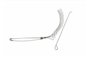
FR150U: Standard Duty, Split Rod, Single Eye, Cable Diameter 1.50 - 1.74 inches, Bale Length 12-in, Mesh Length 18-in, Break Strength 1680 lbs.
