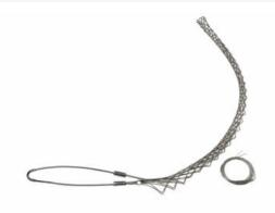
FSHL100U: Heavy-Duty, Split Lace, Single Eye, Cable Diameter 1.00 - 1.24 inches, Bale Length 10-in, Mesh Length 29-in, Break Strength 4720 lbs.
