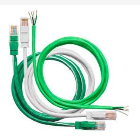
This type of wire connects low voltage devices (i.e., switches, occupancy sensors, photocells) to panels. It is #20 AWG wire that meets UL and NEC standards for Class 2 applications. Plenum rated wire meets plenum and riser requirements. Several types of multiconductor low voltage wires are available for standard, pilot, locator, and multilevel switching or for connecting photocells to the LI control panels. This wire can also be used to wire relays remotely
