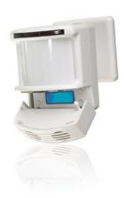
The LMDX-100 Digital Dual Technology Corner Mount Occupancy Sensor uses both passive infrared (PIR) and ultrasonic technologies to achieve precise occupancy sensing for energy-efficient control of lighting and plug loads. It is a digital sensor, and is part of a Wattstopper Digital Lighting Management (DLM) system.
