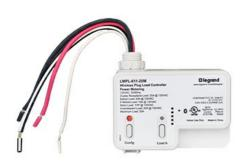
LMPL-611-20M Plug Load Controllers include a 20 amp relay for on/ off control of connected outlets, and a high-efficiency switching power supply. They enable energy-efficient control of plug loads as a part of the Wattstopper Digital Lighting Management (DLM) system.
