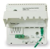
LMRC-210 Series Digital Room Controllers include one, two or three relay(s) to switch a total of 15 or 20 amps, a highefficiency switching power supply and one 0-10 volt output per relay for control of dimmable loads including electronic ballasts (Advance Mark 7, or equivalent). They are the foundation of a Wattstopper Digital Lighting Management (DLM) system, and allow integration of occupancy sensors, daylighting controls and switches for energy-efficient lighting control.
