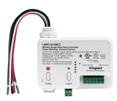
The LMRC-611MCC is a wireless DLM room controller, part of the foundation of the wireless Digital Lighting Management (DLM) system which includes occupancy sensors, daylighting controls, and switches for energy-efficient control. The LMRC-611MCC includes one relay to switch a total of 10 amps, a high-efficiency switching power supply, and both Class 1 and Class 2 0–10 volt outputs for control of dimmable loads including compatible LED drivers and electronic ballasts.
