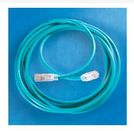
Clarity 6 Modular Patch Cord, blue, 5', Category 6, four-pair UTP stranded 24 AWG PVC/CM, center tuned with Clarity 6 connecting hardware for optimum Category 6 installed performance using Ortronics Paralign 2 pair-positioning technolgy
