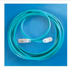
Clarity 6 Modular Patch Cord, blue, 10', Category 6, four-pair UTP stranded 24 AWG PVC/CM, center tuned with Clarity 6 connecting hardware for optimum Category 6 installed performance using Ortronics Paralign 2 pair-positioning technolgy
