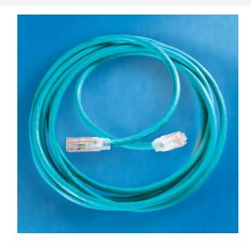
Clarity 6 Modular Patch Cord, blue, 15', Category 6, four-pair UTP stranded 24 AWG PVC/CM, center tuned with Clarity 6 connecting hardware for optimum Category 6 installed performance using Ortronics "Paralign 2" pair-positioning technolgy
