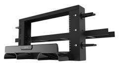
Overhead rack to support additional rack space above existing racks or cabinets. Easily installs to wire cable tray, tubular runway, or threaded rod. The racks are fully assembled and bonded as packaged. The racks are available in 2RU thru 8RU, in black or white to match any installation. Includes a 3 piece waterfall to elegantly route cables down to the lower racks. Used when floor space is at a premium or for easy top of rack cable patching.
