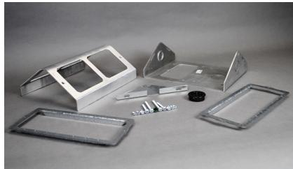
Dual-service fitting includes housing, base, two mounting frames, divider, and mounting hardware. For use on PK, or one No. 2 or one No. 4 Pro Series Duct. Has 1/2" and 3/4" trade size conduit knockouts on each end. 104.3 cu. in. (1709cm3) capacity.
