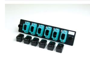
The Ortronics OptiMo® OFP series adapter panels are used with our popular FC Series modular fiber cabinets, offering great flexibility in structured cabling design. Front-removable adapter panels are available with LC, SC, ST, and MT-RJ adapters and feature options ideal for both single mode and multimode applications.
