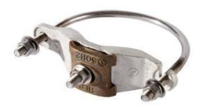
Nominal pipe size range: 3.5" – 4", pipe outside diameter: 3.2" –4.5" Manufactured from electroplated tinned bronze. Conductor range: #6 through 250 MCM PEM stud ensures a flush mounting surface. 5pk.
