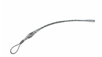
Light Duty, Standard Length, Flexible Eye. Cable Diameter - 2.500-2.990-inch, Mesh Length - 28-inch, Break Strength - 13,000 lbs.
