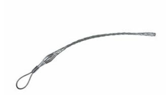
Light Duty, Standard Length, Flexible Eye. Cable Diameter - 3.000-3.490-inch, Mesh Length - 30-inch, Break Strength - 16,200 lbs.
