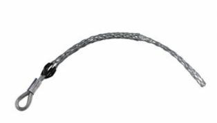
Medium Duty, Short Length, Flexible Eye, T-Type. Cable Diameter -1.500-1.990-inch, Mesh Length - 24-inch, Eye Diameter - 7/16-inch, Break Strength - 16,400 lbs.
