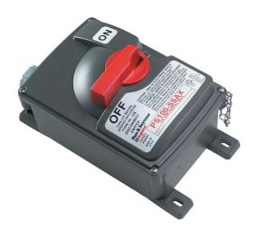
Non-Fusible Safety Switch with Auxiliary Contact, 100 Amps, 600 VAC. The first non-metallic NEMA 4X Non-Fusible Safety Switch line UL Listed as Suitable as Motor Disconnect per NEC Article 430.109(A)(6). Pass and Seymour Non-Fusible Safety Switches feature extra-tough components, including an impact-resistant Valox NEMA 4X enclosure. And an innovative design that delivers safe, sure operation under the worst conditions.
