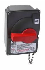
Non-Fusible Safety Switch with Auxiliary Contact, 30 Amps, 600 VAC. The first non-metallic NEMA 4X Non-Fusible Safety Switch line UL Listed as Suitable as Motor Disconnect per NEC Article 430.109(A) (6). Pass and Seymour Non-Fusible Safety Switches feature extratough components, including an impact-resistant Valox NEMA 4X enclosure. And an innovative design that delivers safe, sure operation under the worst conditions.
