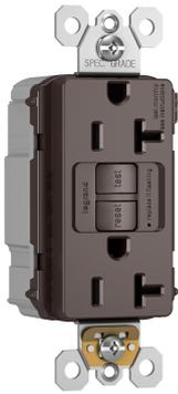
PlugTail® Spec-Grade Tamper-Resistant 20A Self-Test Duplex GFCI. Self-test GFCI Technology - conducts an automatic test every three seconds, ensuring it's always ready to protect. PlugTail® devices and connectors mean that device installation is the same regardless of skill level of the installer. The UL-Listed connectors are keyed to ensure proper wiring installation into each receptacle.
