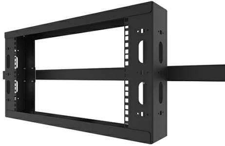
Overhead rack to support additional rack space above existing racks or cabinets. Easily installs to wire cable tray, tubular runway, or threaded rod. The racks are fully assembled and bonded as packaged. The racks are available in 2RU thru 8RU, in black or white to match any installation. Used when floor space is at a premium or for easy top of rack cable patching.
