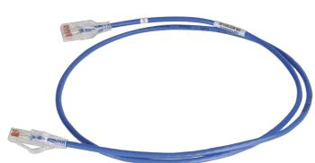
RDC610 Modular Patch Cord, blue, 8', reduced diameter, 28 AWG, cat6a channel four-pair UTP stranded PVC/CM.
